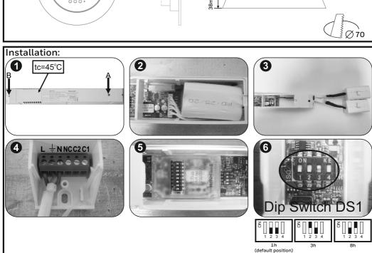
To install this luminaire, a hole  $\varnothing$  70 mm must be cut in the suspended ceiling. For correct mounting, observe the light direction. **Step 1:** Unfasten the mounting screws, **A** for battery compartment and **B** for electrical connections. Remove the respective covers. **Step 2:** Connect the battery and place the battery inside the compartment. Refit the cover and fasten the removed screw (**A**) in step
