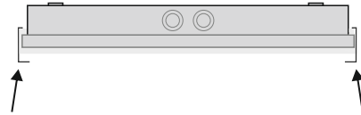
Step 2: Place the holding accessories to the luminaire.
